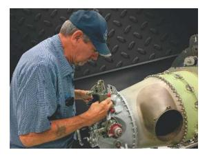
If budgeting, \$30,000 would be a good average. This includes overhaul or replacement of the CT Vane Ring. PT6A CT Vane Rings are prone to inner and outer support cracking.
